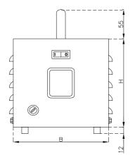
Enclosures EO 23 are designed for mounting of single phase transformers with rated power up to 1 KVA.
